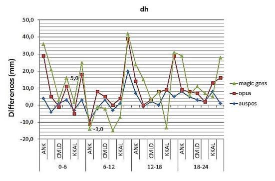
Figure 4: The differences of coordinates components for 6 hour data
