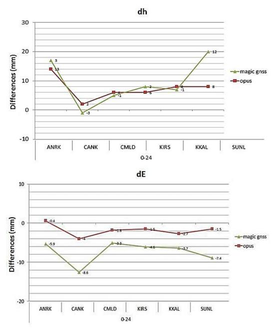
Figure 2. The differences between coordinates components for 24-hour data obtained by taking AUSPOS as a reference
