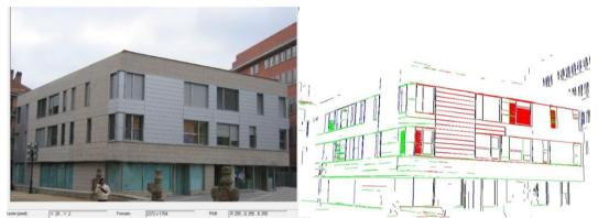
Fig. 7: Original single image (left), segmentation and clustering of vanishing lines (right)
