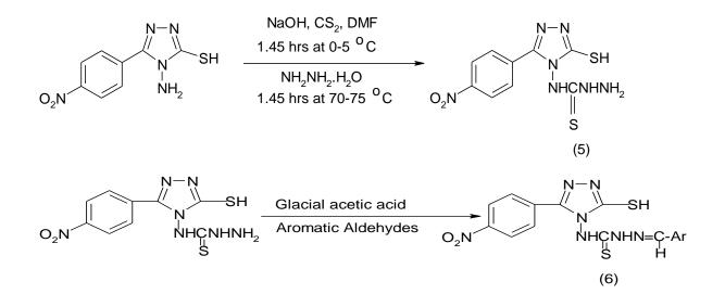
IR (KBr, cm<sup>-1</sup>): 3276.83(NH<sub>2</sub>),1504.37(C-NO<sub>2</sub>) 1618.17(C=N),1309.58(C=S),1188.07(C-N C),1269.07(C=S),3093,2920.03 (-CH),1477.37(C-C), 1677.95(-CSNH)
