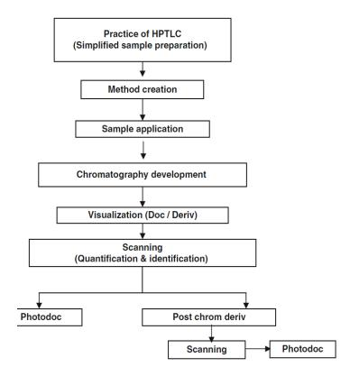
Figure 1: Schematic diagram of HPTLC method of separation
