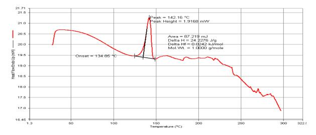
Figure 5: DSC Thermogram of formulation
