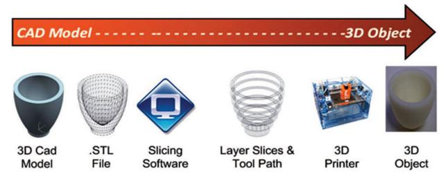
Fig. 1. The process of 3D-printing (13)
