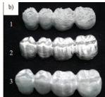
Fig. 3. Wax patterns, produced by 3D printing – a) and 4-part bridges produced by SLM of Co-Cr alloy – b). (1 – as received SLM bridge, 2 – after mechanical treatment, 3 – after sand-blasting)
