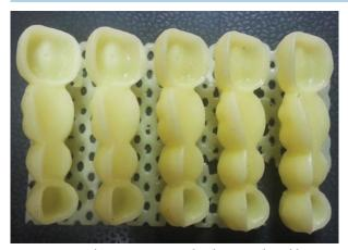
Fig. 4. Polymer temporary bridges, produced by stereolytography.
