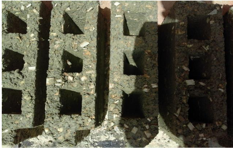
Figure 1: Bricks hollow block containing typha australis ( c/g=0.2 )
