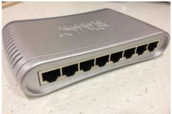
Figure 6: SMCFS8 Ethernet Switch
