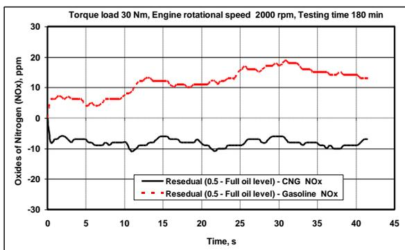
Figure 3: Residual values of oxides nitrogen (NO<sub>x</sub>) for gasoline and CNG
