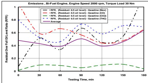
Figure 12: Average RFR exhaust emission component for gasoline phase
