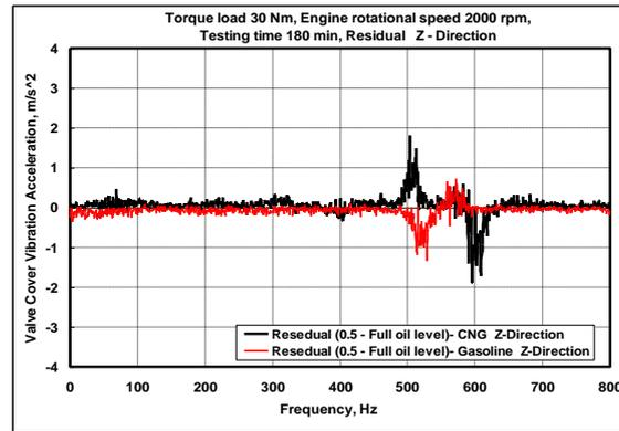
Figure 9: Residual vibration acceleration for gasoline and CNG in Z-direction
