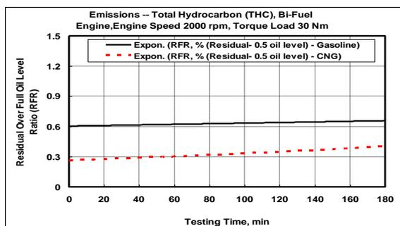
Figure 10: RFR exhaust emission for gasoline and CNG in THC component
