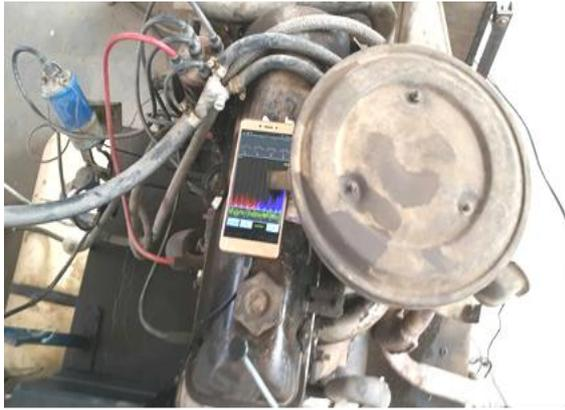
Figure 1: Vibration sensor position overview
