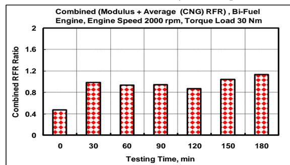
Figure 17: Combined RFR CNG engine phase
