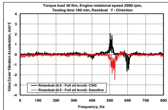
Figure 8: Residual vibration acceleration for gasoline and CNG in Y-direction
