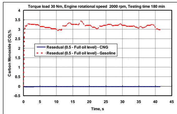
Figure 4: Residual values of carbon monoxide (CO) for gasoline and CNG
