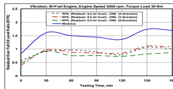
Figure 15: Modulus RFR engine vibration acceleration (X,Y,Z) for CNG phase
