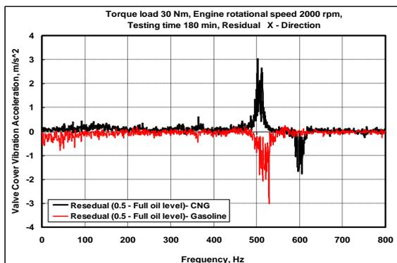
Figure 7: Residual vibration acceleration for gasoline and CNG in X-direction
