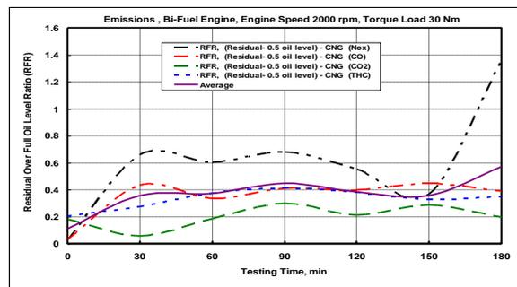
Figure 13: Average RFR exhaust emission component for CNG phase
