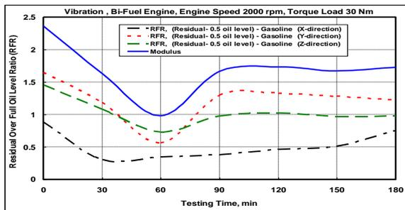
Figure 14: Modulus RFR engine vibration acceleration (X,Y,Z) for gasoline phase
