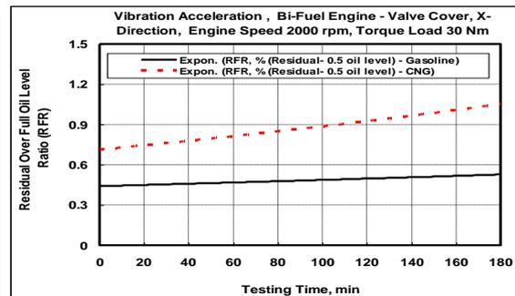
Figure 11: RFR vibration acceleration for gasoline and CNG in X-direction
