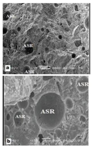
Figure 3: ASR products monitored via SEM
