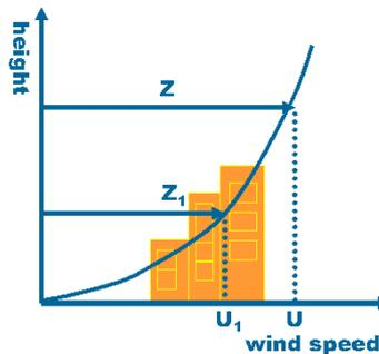
Figure 4: Vertical wind profile in the atmospheric boundary layer
