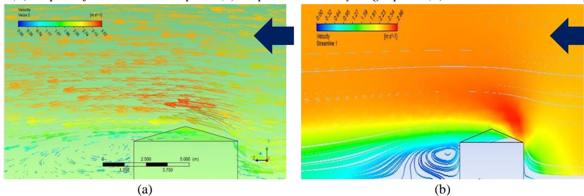
Figure 8: Air flow from front towards back side of house: (a) Velocity vector YZ plane front window central plane (b) streamline velocity YZ plane central plane
