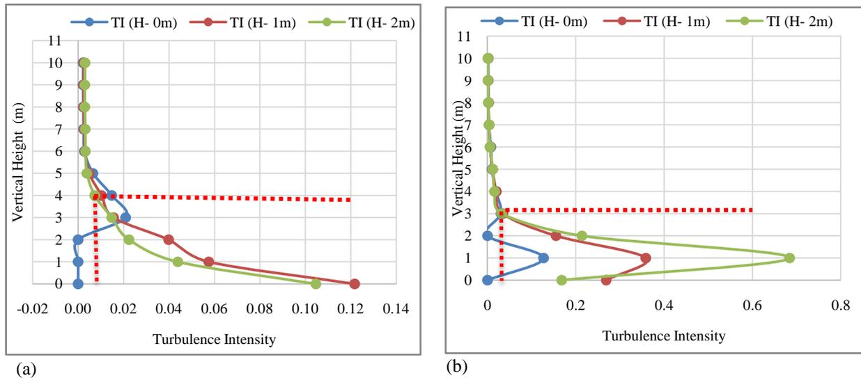
Figure 9: Turbulence intensity distribution: a) turbulence intensity on windward (front part) of house; b) turbulence intensity on leeward side (back part) of house
