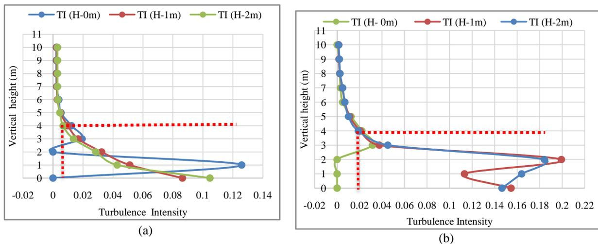
Figure 12: Turbulence intensity distribution: a) turbulence intensity windward side (front part); b) turbulence intensity leeward side (back part)
