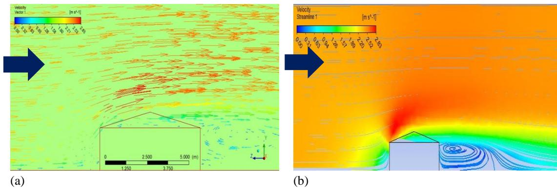
Figure 12: Air flow from back part to front part of the house: (a) velocity vector YZ plane central plane (b) streamline velocity YZ central plane
