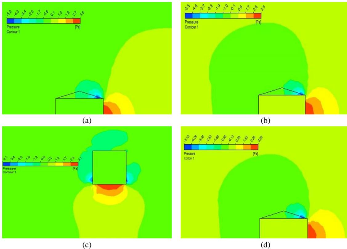
Figure 7: Air flow from front to back part of house: Pressure contour (a) YZ plane front window central plane (b) YZ plane front door central plane (c) XZ plane at chimney height plane (d) YZ back window central plane
