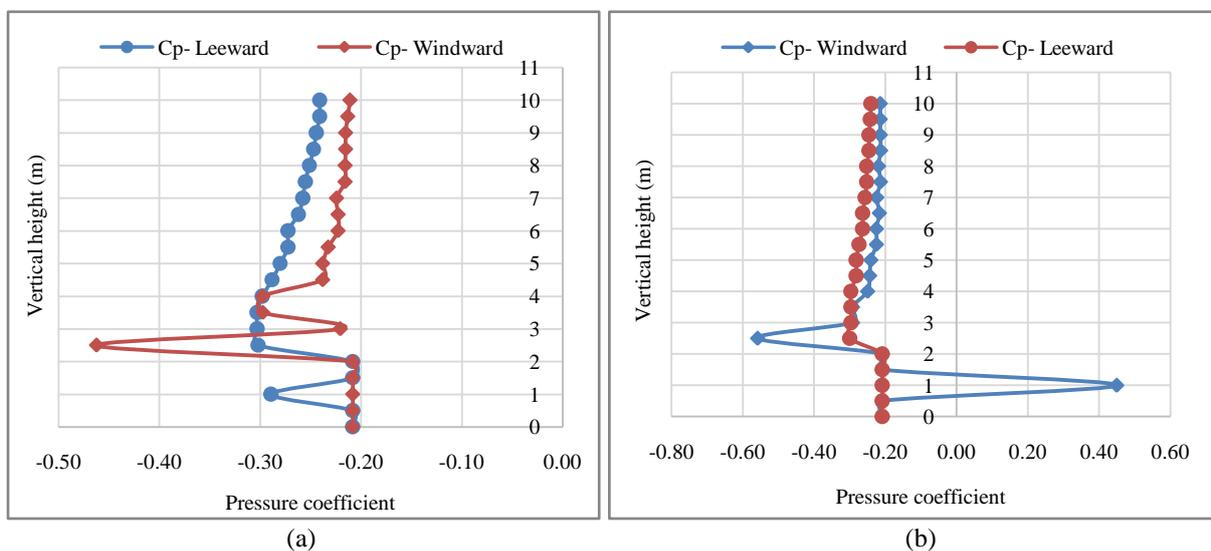
Figure 6: Pressure coefficient distribution at different vertical height: (a) Pressure coefficient at different points while wind flow from front part (b) Pressure coefficient at different location while wind flow from back part.
