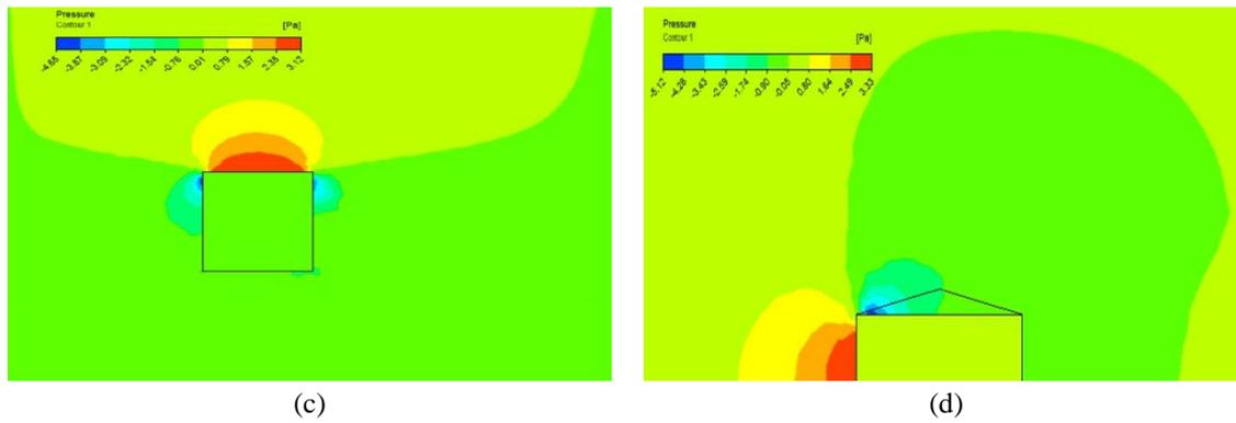
Figure 10: Air flow from back to front part of house- pressure contour: (a) YZ plane front window central plane (b) YZ plane front door central plane (c) XZ plane at chimney height plane (d) YZ back window central plane
