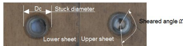
Figure 8: Indication of angular shear nugget
