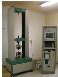
Figure 4: The universal type tensile test machine ETI-E0015
