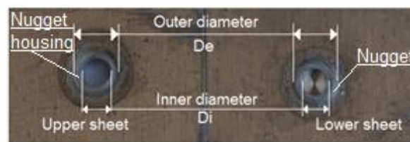
Figure 7: Indication of D_e and D_i nugget
