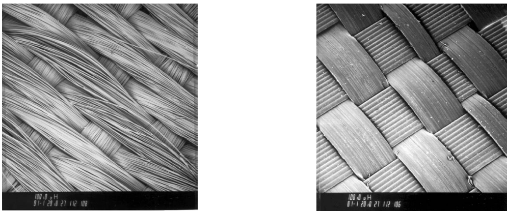
Figure 1: Plan view photomicrographs of woven geotextiles: (a) multifilament fiber (magnified 8×); (b) slit-film fiber (magnified 8×)
