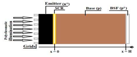
Figure 1: Silicon solar cell n+pp+ type
