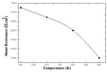
Figure 6: Shunt resistance as a function of temperature
