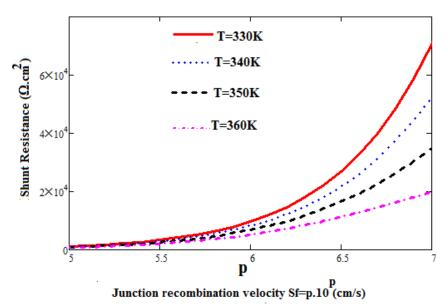
Figure 7: Shunt resistance as a function of the recombination rate at the junction for different temperature values
