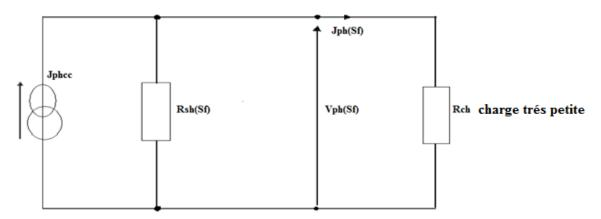
*Figure 6: Electrical equivalent circuit of the solar cell unit when it operates practically in short-circuit* Using the circuits of figure 6, the shunt resistances can be expressed as:
