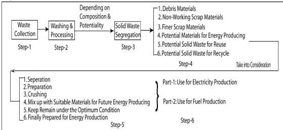
Figure 4: Shows the possible pathway to engergy producing technique using solid waste
