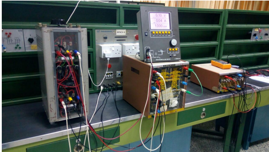
Figure 17: Three-phase Transmission Line Impedance Test Fault
