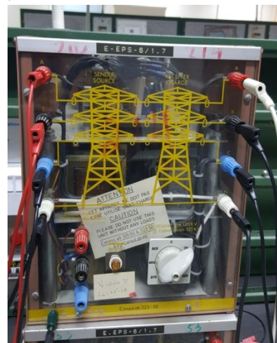
Figure 9: Equivalent transmission line circuit
