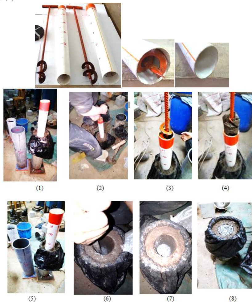
Figure 3: Steps of pile installation and the PVC pipes
