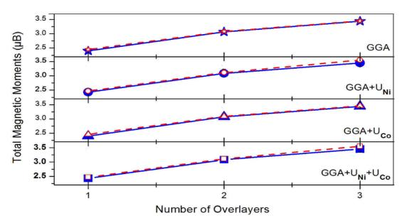
Figure 2: Total magnetic moments of  $Ni_n/Co$  (111) orientation for n = 1-3 overlayers. Solid symbols straight lines for relaxed and open symbols dotted lines for non-relaxed. Star for GGA, Circle for GGA+ $U_{Ni}$ , triangle for GGA+ $U_{Co}$  and Square for GGA+ $U_{Ni}+U_{Co}$  respectively.
