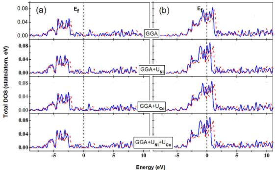
Figure 6: Total DOS of  $Ni_n/Co$  (111) orientation for (a) n=1 and (b) n=3 overlayers, for GGA, GGA+ $U_{Ni}$ , GGA+ $U_{Co}$  and GGA+ $U_{Ni}+U_{Co}$  respectively. Solid lines for non-relaxed and dashed lines for relaxed cases.
