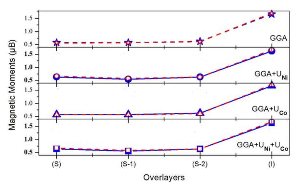
Figure 1: Magnetic moments of three-layers for  $Ni_n/Co$  (111) orientation. Solid symbols straight lines for relaxed and open symbols doted lines for non-relaxed. Star for GGA, Circle for GGA+ $U_{Ni}$ , triangle for GGA+ $U_{Co}$  and Square for GGA+ $U_{Ni}+U_{Co}$  respectively.
