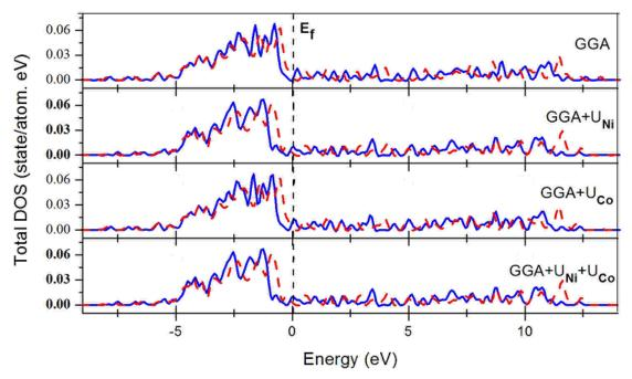
Figure 5: Total DOS of  $Co_n/Ni$  (111) orientation for n = 2 overlayers, for GGA, GGA+ $U_{Ni}$ , GGA+ $U_{Co}$  and  $GGA+U_{Ni}+U_{Co}$  respectively. Solid lines for non-relaxed and dashed lines for relaxed cases.
