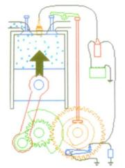
Figure 2: a diagram showing the compression stroke
