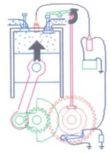
Figure 4: a diagram showing the exhaust stroke
