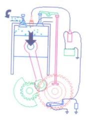
Figure 1: A diagram showing the intake stroke.
