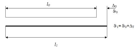
*Figure 6: Change in length of a rod due to thermal expansion.*
