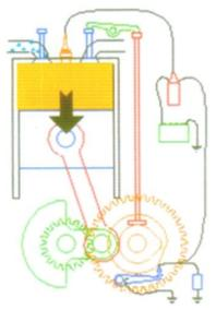
Figure 3: a diagram showing the power stroke
