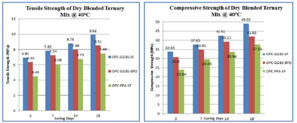
*Figure 2: The summary of results of Split tensile and Compressive strength test of the 50mm*× 50 mm Ternary blended mix cured at elevated temperature @ 40 °C.
