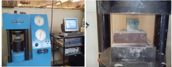
Plate 3: Split Tensile and Compressive Strength Test.
