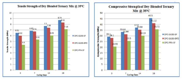
*Figure 3: The summary of results of Split tensile and Compressive strength test of the 50 mm*× 50 mm Ternary blended mix paste cured at elevated temperature @ 35 °C.
