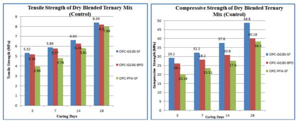
Figure 1: The summary of results of Split tensile and Compressive strength test of the Control 50 mm× 50 mm Ternary blended mix.
