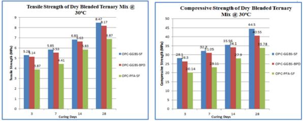
*Figure 4: The summary of results of Split tensile and Compressive strength test of the 50 mm*× 50 mm Ternary blended mix paste cured at elevated temperature @ 30 °C.
