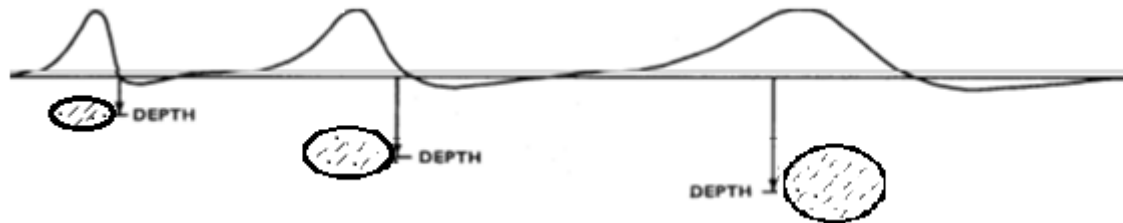
Figure 17: Effect of Depth on Anomaly Shape and Amplitude([modified from 18]).
