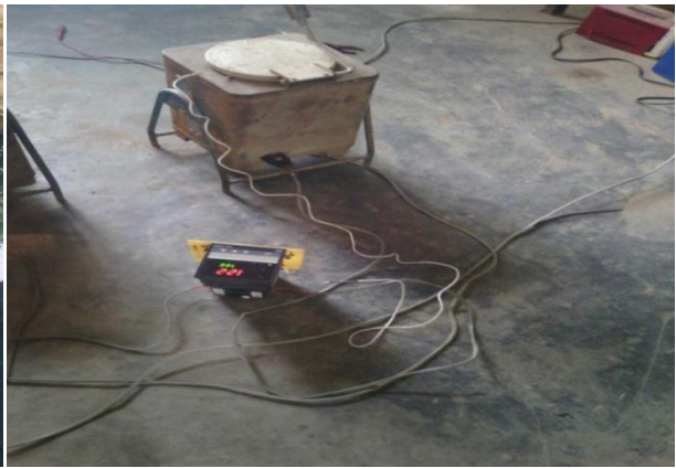
Plate 4: Connection of the thermocouple, temperature controller and the contactor
