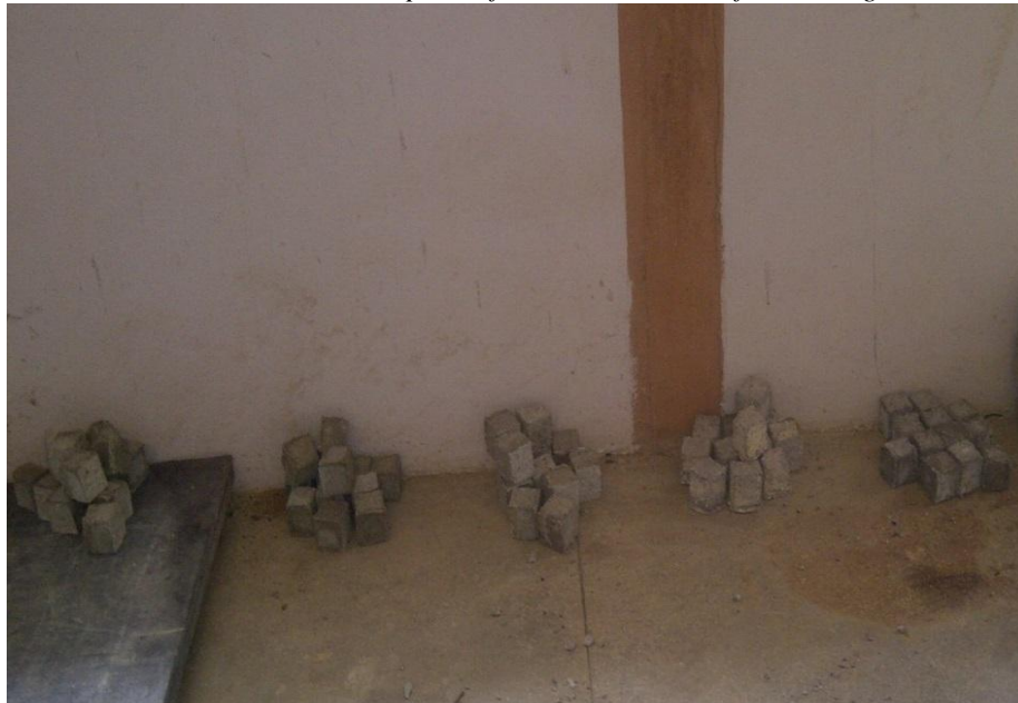
Plate 5: The removed cubes from the pallet according to different percentages of glass fibre
