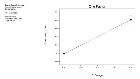
Figure 4: Model graph of concentration Vs dosage for PTSC
