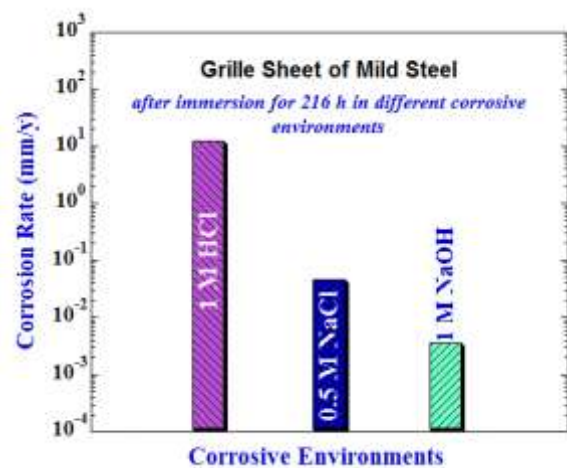
Fig. 1: Corrosion rate of the mild steel sheet in 1 M HCl, 0.5 M NaCl and 1 M NaOH solutions open to air at 25\pm 1^\circ\text{C}
