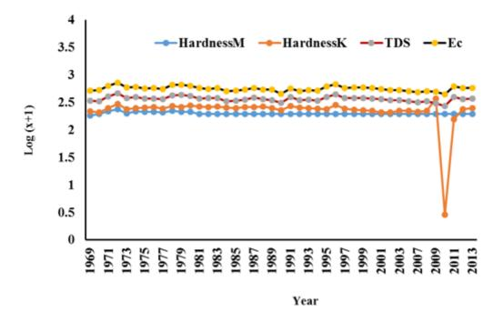
**Fig. 5:** Changes in parameters of Total and Temporary Hardness, Dissolved Solids and Electrical Conductivity of the Neka River.
