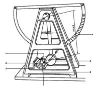
Figure 2. Lateral impact tester (ISO 19953)
