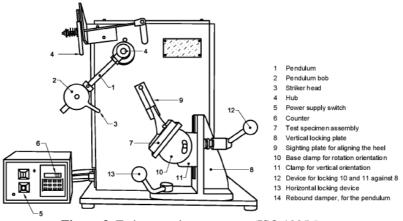
Figure 3. Fatigue-testing apparatus (ISO 19956)
