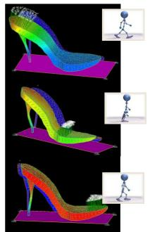
Figure 13. FEM simulation of shoe and heel strain reactions under simplified load conditions
