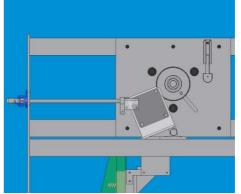
Figure 9. Pivoting motor and anti-rebound system
