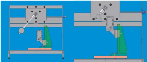
Figure 10. Equipment with double configuration, used for single impact (up) or fatigue tests (down) by acting on pendulum's dimension, fixture and alignment system
