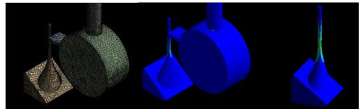
Figure 14. FEM dynamic simulation of impact of pendulum on heel
