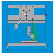
Figure 5: Frontal view with pendula and alignment system
