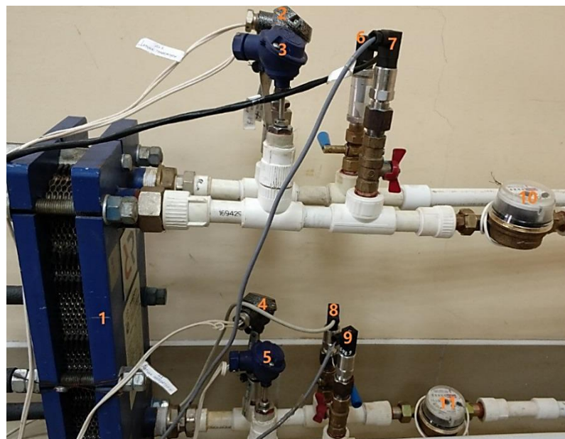
Figure 4. Experimental test section—plate heat exchanger; 2, 3, 4, 5 — M5100 pressure transmitters; 6, 7, 8, 9 — thermometers; 10, 11 — mechanical flow meters
