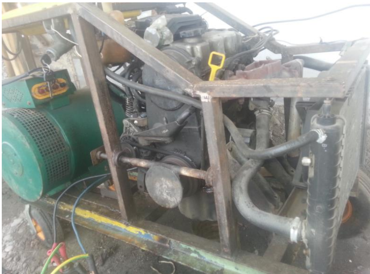
Figure 4. The developed source of electric energy on the basis of ICE the car of mark MATIZ.
