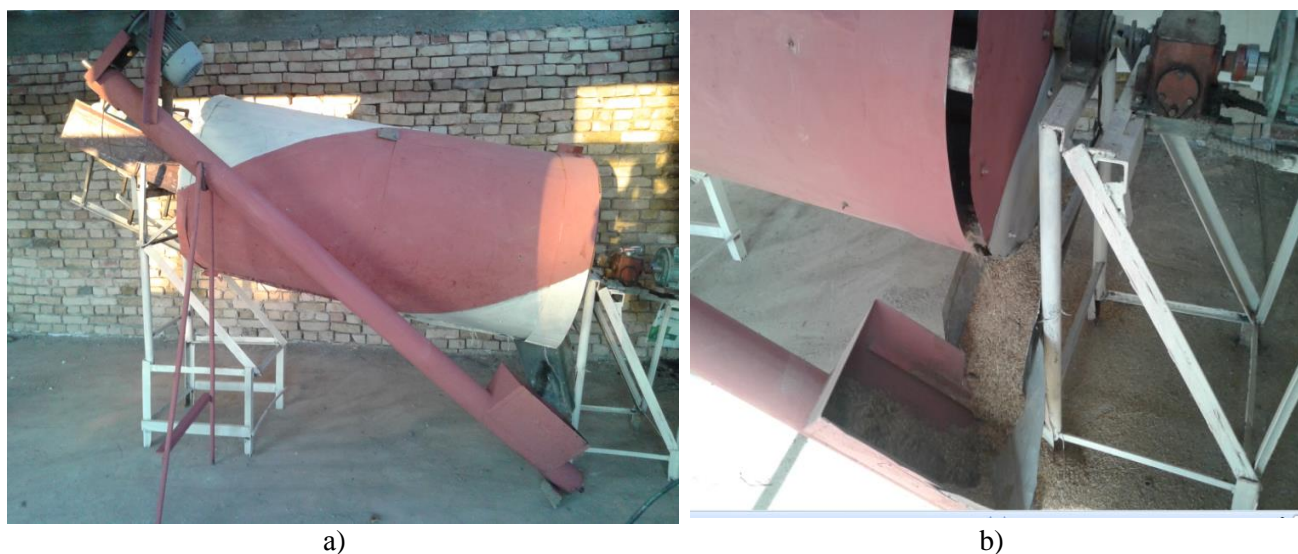
Figure 1. An initial pre-production model of the device for drying of the products of grain crops: a) general view; b) kind of the nutritious bunker and a trench
