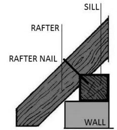
Fig. 4. The scheme of the rafter-wall connection
