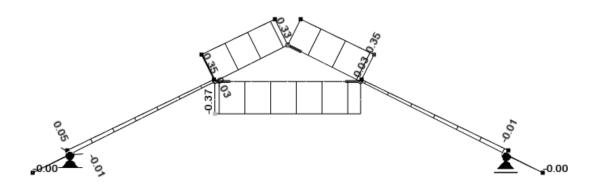
Fig. 3. The static scheme and the distribution of the axial forces [kN] of the rafter – doubled collar tie system
