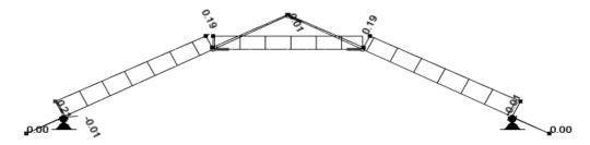
Fig. 2. The static scheme and the distribution of the axial forces [kN] of the rafter – collar tie system
