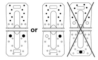
Fig. 10. The schematic examples of arrangements of the nails and screws [8]
