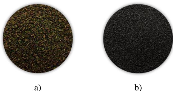
Fig.4. Elastomer phase derived rubber types a) rubber granules; b) rubber powder
