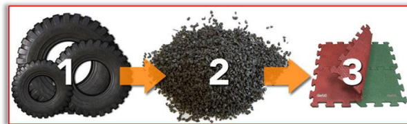
Fig.8. Steps to obtaining the rubber flooring
