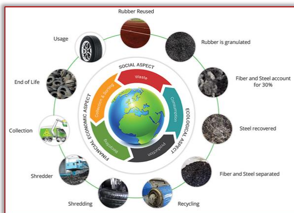
Fig.7. Tire recycling: From waste to final product
