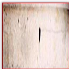
Fig.2. Heat cracks (P=0.134%), appeared during at the thermal treatment
