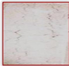
Fig.1. Heat cracks (P = 0.139%), appeared during at the thermal treatment
