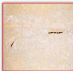
Fig.2. Heat cracks (P=0.134%), appeared during at the thermal treatment
