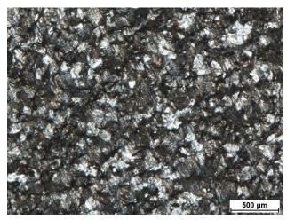
Fig. 2. Surface morphology of AZ31 after DCPD electrodeposition
