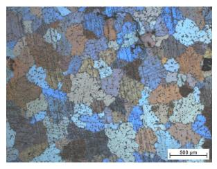
**Fig. 1.** Microstructure of AZ31 magnesium alloy, light microscopy, etch. picric acid + ac. acid + ethanol + water
