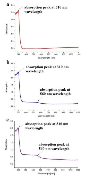
**Fig. 2** UV-Vis spectrum obtained for nanofibers a) PAN polymer, b) PAN5%/Fe<sub>2</sub>O<sub>3</sub> composite c) PAN/10%Fe<sub>2</sub>O<sub>3</sub> composite.
