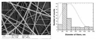
Fig. 3. The SEM image of the obtained PVP nanofibers for sample no 2 and histogram showing the values of nanofibers diameters
