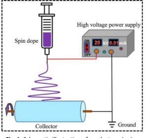
Fig. 1. Schematic illustration of an electrospinning process [18]
