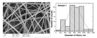
**Fig. 2.** The SEM image of the obtained PVP nanofibers for sample no 1 and histogram showing the values of nanofibers diameters
