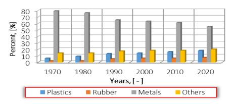
Fig. 2. Change in vehicle composition from 1970 to 2010 [8]
