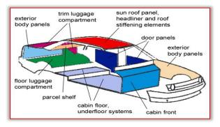
Fig. 4. Potential applications in automotive parts [4]
