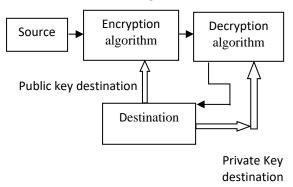
Fig. 3. Asymmetric Key Cryptography
