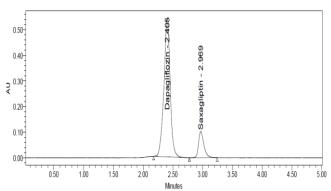
Fig. 10: Flow minus chromatogram of Dapagliflozin and Saxagliptin
