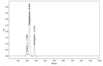
Fig. 13: Base chromatogram of Dapagliflozin and Saxagliptin
