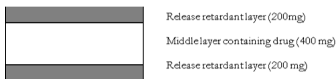
Fig. 1: Approach of three layer matrix tablet
