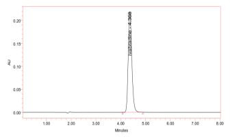
Fig. 3: Typical chromatogram of ivabradine hydrochloride from sample solution
