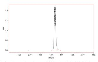
Fig. 2: Typical chromatogram of ivabradine hydrochloride from standard solution
