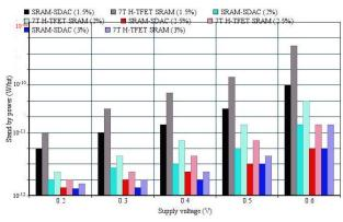
Figure.7 Standby power comparison with varying supply voltage
