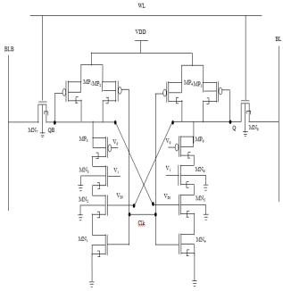
Figure.3 SRAM cell with d-INDEP logic
