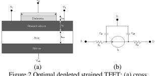
Figure.2 Optimal depleted strained TFET: (a) cross section and (b) equivalent circuit
