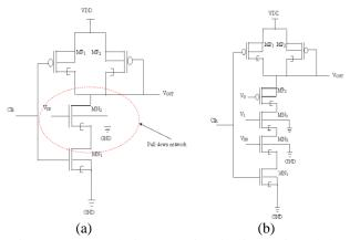
Figure.1 Inverter design: (a) using domino logic and (b) using d-INDEP logic
