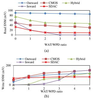
Figure.5 SNM of: (a) read and (b) write operation with 0.3 V
