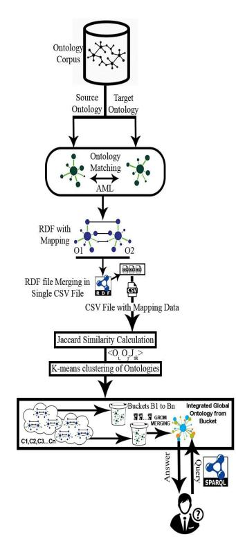
Figure. 1 Flow diagram of the proposed system
