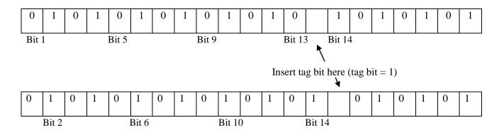
Figure.4 Inserting tag bits after bit 13 and bit 14
