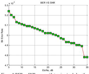
Figure.8 BER vs SNR curve with tagging (code length = 1000 bits, QPSK)
