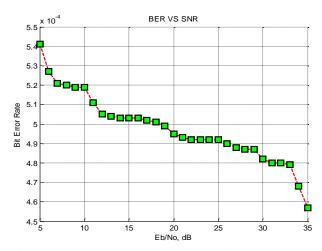
Figure. 6 BER vs SNR curve with tagging (code length = 1000 bits, BPSK)
