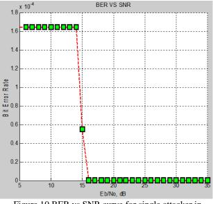
Figure.10 BER vs SNR curve for single attacker in network
