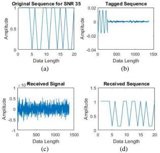
Figure.5 Signal of 20 bits transmitted using tagging and chaotic communication
