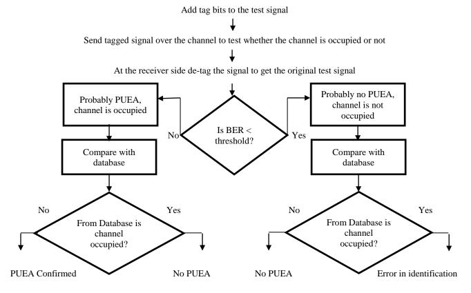
Figure.11 Flowchart showing the entire proposed method to detect PUEA
