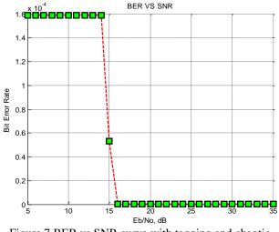
Figure.7 BER vs SNR curve with tagging and chaotic communication (code length = 1000 bits, BPSK)
