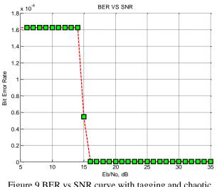
Figure.9 BER vs SNR curve with tagging and chaotic communication (code length = 1000 bits, QPSK)
