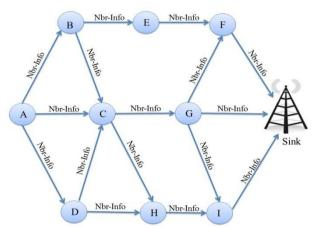
Figure.1 Sensors send the Nbr-Info packet to the sink
