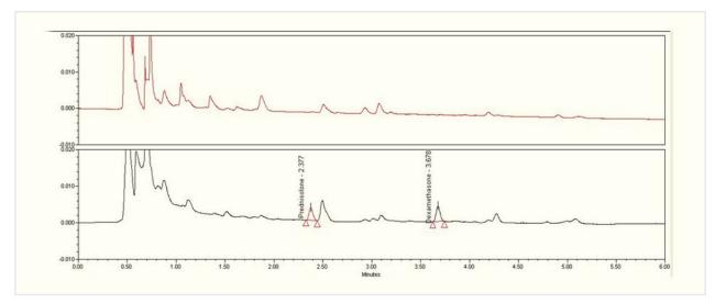
**Fig 3.** The chromatograms of extracted (A) blank plasma, (B) plasma spiked with 50 ng/mL of dexamethasone and IS.
