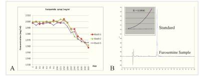
**Fig 1A.** Change in concentration of furosemide in furosemide syrup 2 mg/ml when stores for 360 days at 2-8°C. **Fig 1B.** UPLC chromatogram of the drug analyzed.
