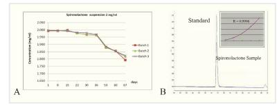
**Fig 2A.** Change in concentration of spironolactone in spironolactone suspension 2 mg/ml when stores for 67 days at 2-8°C. **Fig 2B.** UPLC chromatogram of the drug analyzed.
