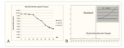
**Fig 3A.** Change in concentration of hydrochlorothiazide in hydrochlorothiazide suspension 10 mg/ml when stores for 34 days at 2-8°C. **Fig 3B.** UPLC chromatogram of the drug analyzed.
