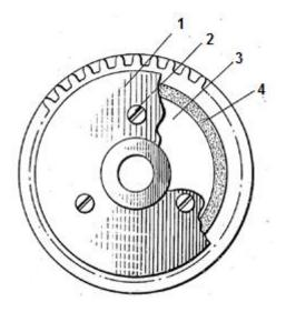
Fig. 7. Scheme of construction of wheel with a malleable ring. Description of indications: 1) side discs; 2) screw connection; 3) wheel hub; 4) susceptible ring [11]
