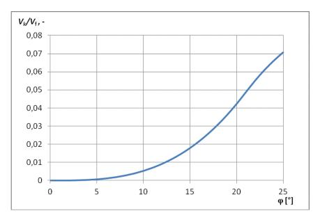
Fig. 6. Graph of Vk/Vf ratio as a function of the angle of hub deflection  $\varphi$
