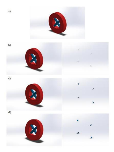
Fig. 3. Simulation of the hub oscillating operation: a) three-dimensional model of the joint showing the main characteristics of the analysed solution; b) the angle between the journal axis and the hub axis is 1°; c) the angle between the journal axis and the hub axis is 5°;d) the angle between the journal axis and the hub axis is 15°
