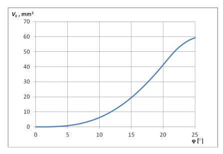
Fig. 4. Overlapping volume Vk diagram as a function of angle  $\phi$  between the journal axis and the hub axis
