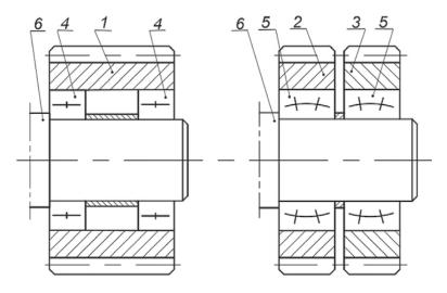
Fig. 1. Diagram of a portion of a satellite wheel with bearing. Description of indications:
