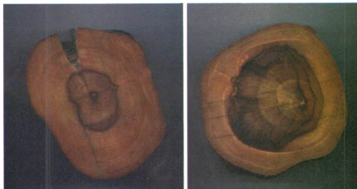
Gambar 1. Penampang lintang kayu JPP (kiri) dan kayu jati konvensional (kanan) Figure 1. Cross section of JPP (left) and the conventional teak woods (right)
