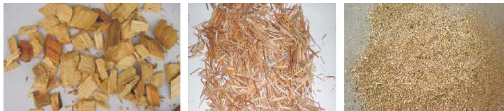
Gambar 3. Macam bentuk dan ukuran chips hasil pengolahan pembuat serpih Figure 3. Size and types of chips produced by chipper
