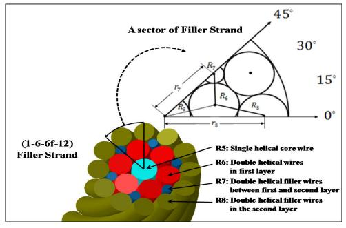
**Figure 2.** (1-6-6f-12) Wire Filler Strand Radiuses and a Sector of Filler Strand
