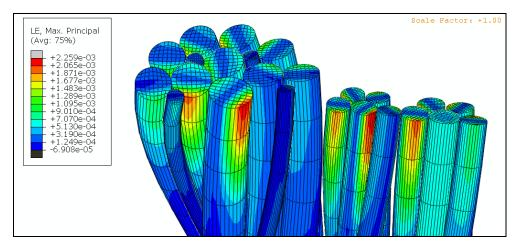
Figure 4. Logarithmic Strain Components Along Filler IWRC on Selected Wires
