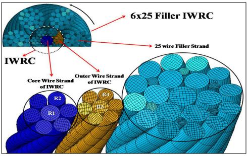
Figure 1. Composition of the 6X25 Filler IWRC Structure
