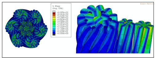
Figure 3. Von-Misses Stress Distribution Along Filler IWRC
